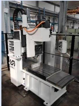
Axial-Torsional Fatigue Tests, Very-High-Cycle Fatigue
